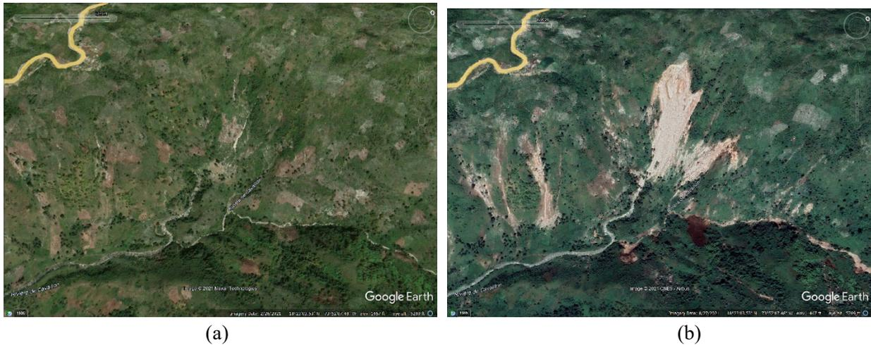
**Figure 7.41.** Landslide near RN7 with an average slope 47% over length of ~0.4 km as measured in Google Earth (18.385256, Lon: -73.869594). (a) February 26, 2021. (b) August 27, 2021.
